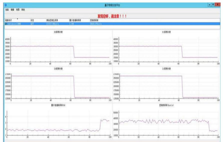
Fig.3 Detection results when QKD is attacked
